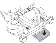
5 Adjust the unit's ground pressure by screwing in or out the adjusting screws located behind the front wheels on both sides. The ground pressure should be between 12 and 15 kg (26.5-33 lb).
